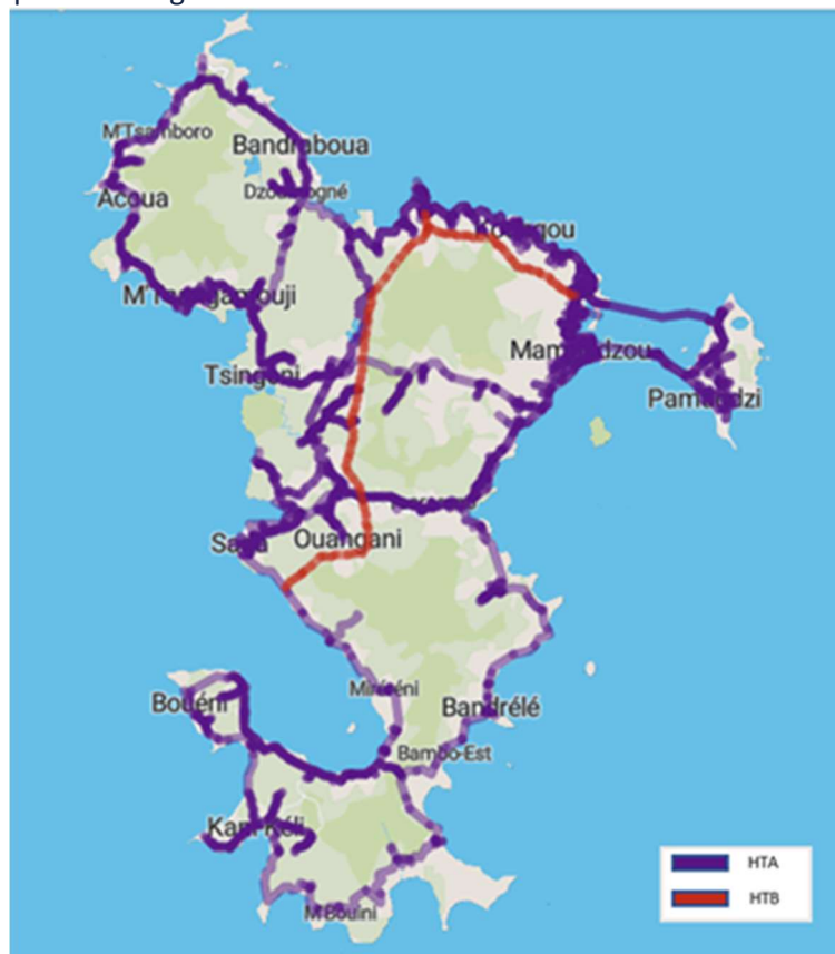
Figure 27: HTA and HTB transmission lines (source: EDM Open Data)
